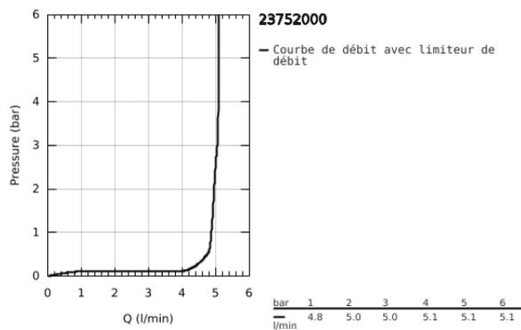
23 752 000 **BAUFLOW MITIGEUR MONOCOMMANDE, 1/2"**
