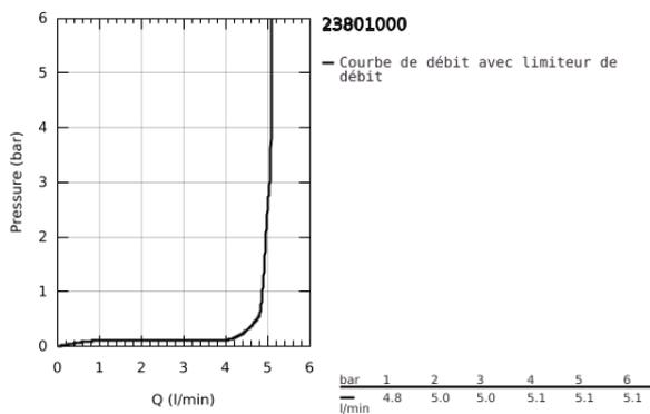
23 801 000 **BAUFLOW MITIGEUR MONOCOMMANDE, 1/2"**
