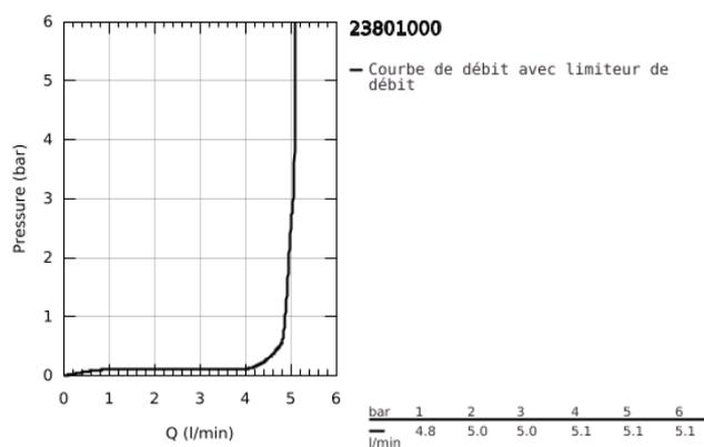
23 801 000 **BAUFLOW MITIGEUR MONOCOMMANDE, 1/2"**
