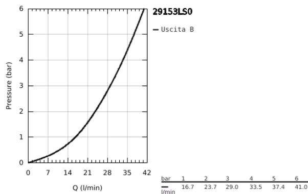
29 153 LS0 **GROHTHERM SMARTCONTROL MISCELATORE TERMOSTATICO A 1 VIA**
